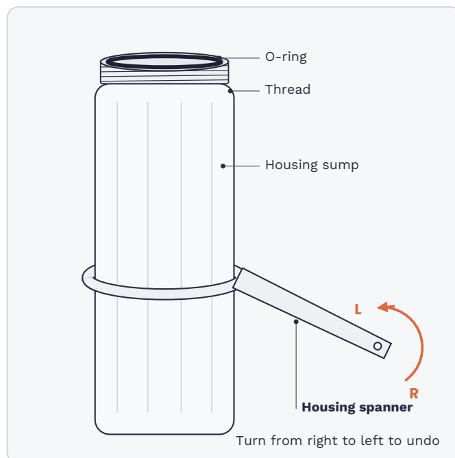
DIAGRAM 3 Removing a housing sump
